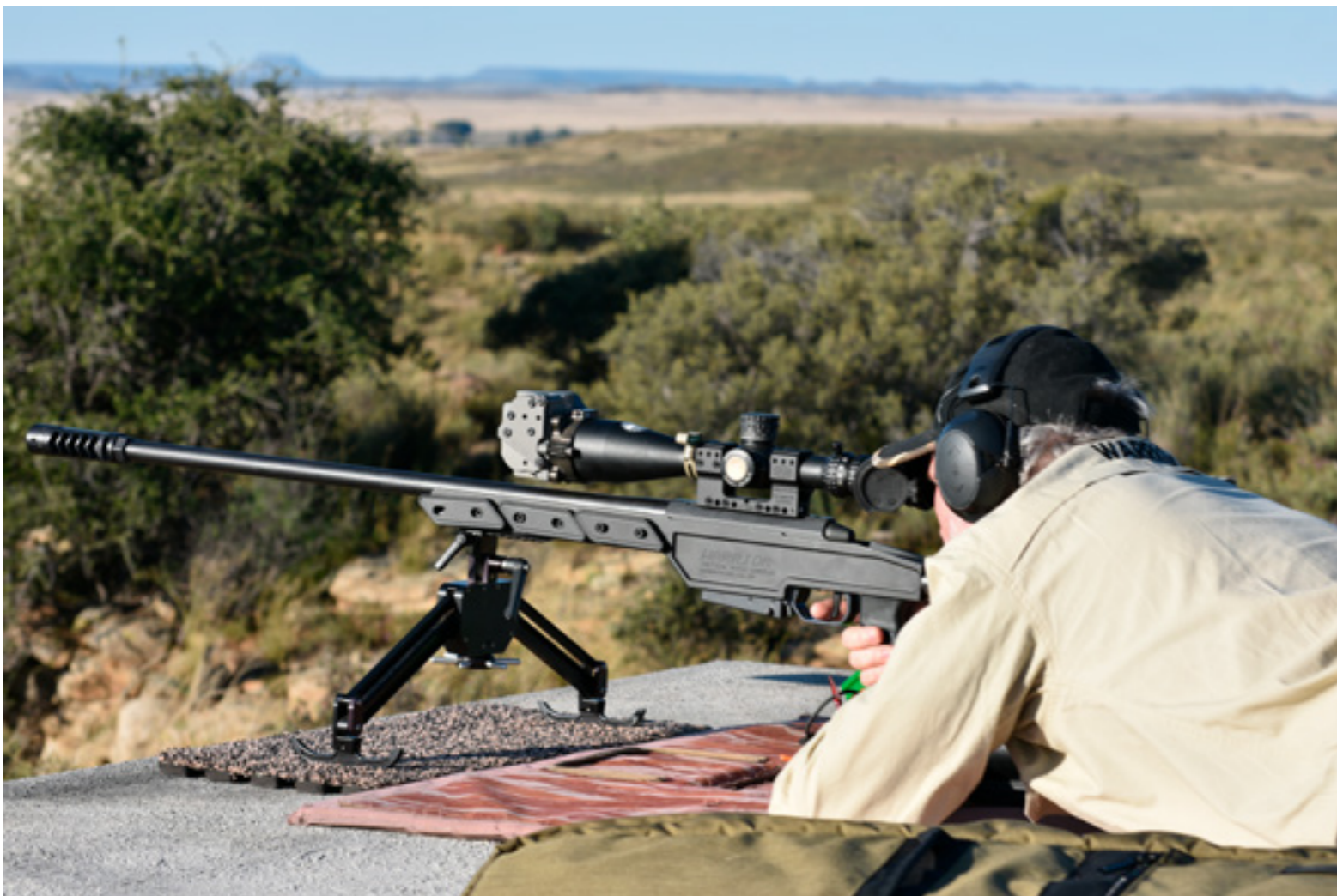
Etienne de Beer taking aim at the 3272 m target. He used a Charlie Tarac to gain additional elevation from a Sako TRG in 338 LM with a Warrior Gen 6 Chassis and Warrior Beast 40 EC tuner brake. His rifle firing 300 gr Berger Tactical OTM bullets. The rifle was built by Warren Britnell and Jurgens Nezar.
